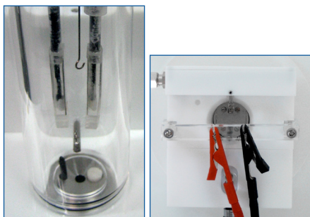
stimulation electrodes on bath (left) and myograph (right), on emkaBATH4 system
