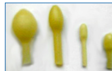
4 sizes of latex balloons for LVP measurement - 7mm X 10mm, 4mm X 8mm, 3.5mm X 5mm and 1.5mm X 3mm
